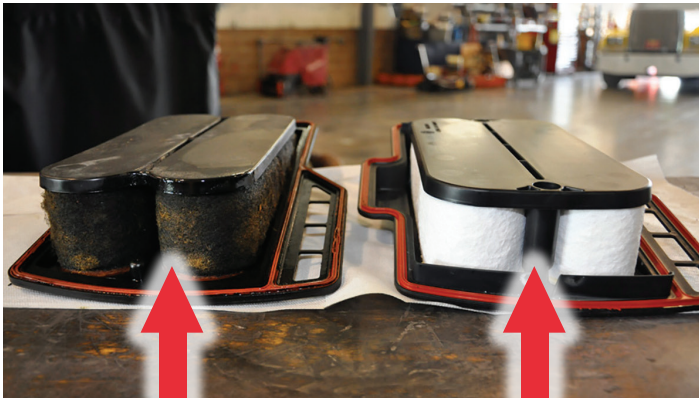
CLOGGED CCV FILTER
